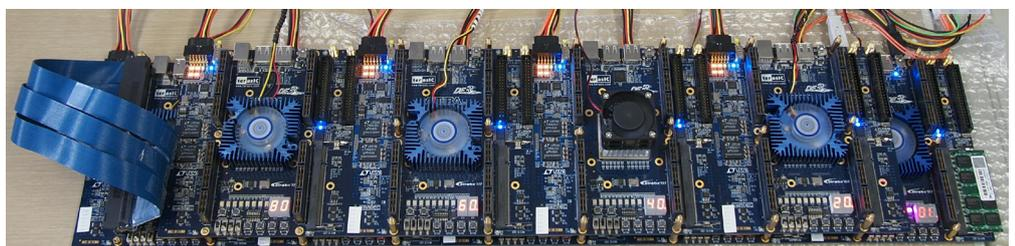
SSA prototyped on nine ALTERA StratixIII FPGAs
