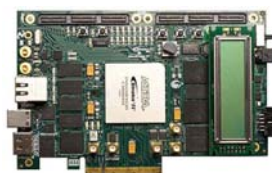
FPGA-based data- compressor
