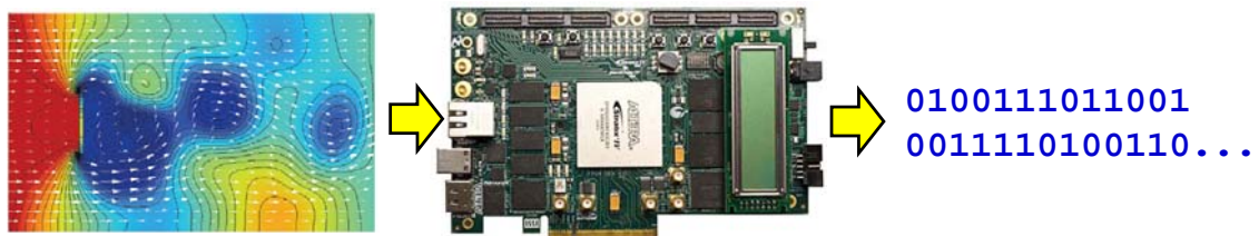
FPGA-based data compressor
